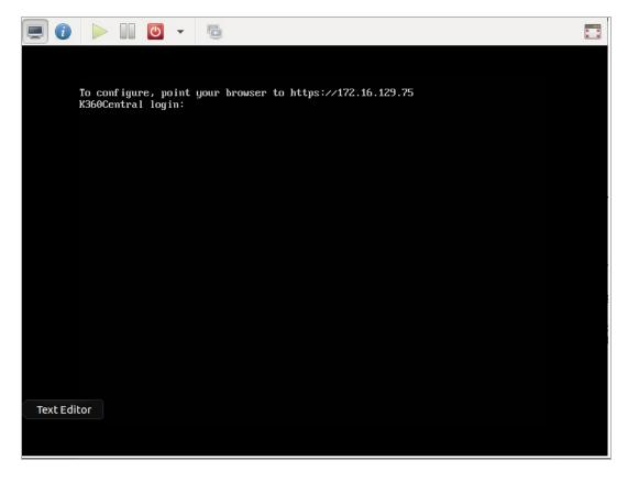
The VM should obtain an IP address using DHCP. Make a note of this address.
