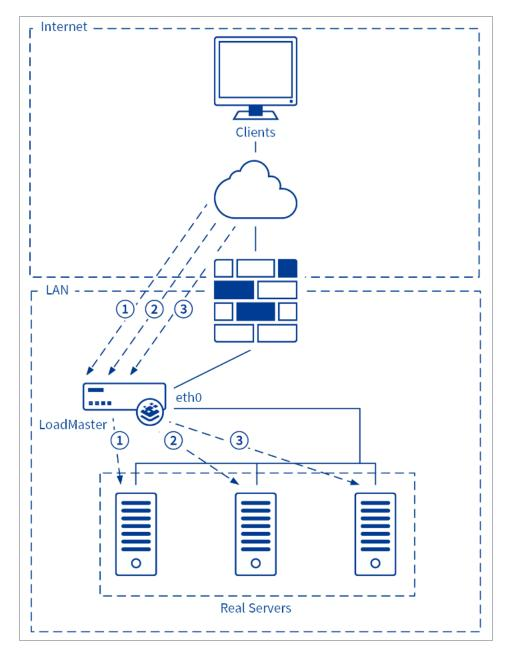
With persistence, the LoadMaster will direct new connections according to the load balancing algorithm, but returning connections will go to the same server (diagram below).
