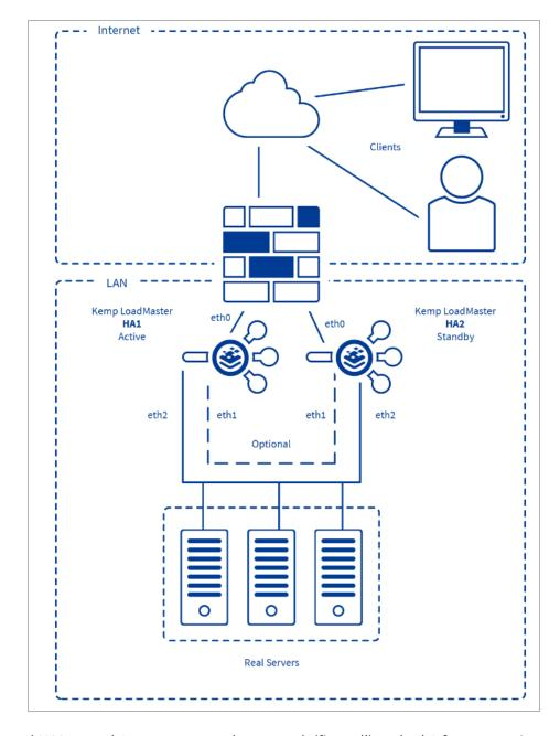
Both HA1 and HA2 use eth0 to connect to the network (firewall) and eth2 for connection to the servers. The two eth0 ports have one shared IP address and the two eth2 ports have a different shared IP address. Health checking between the two LoadMasters occurs between both eth ports. Optionally, eth1 on each unit may be directly connected using a patch cable for added HA health checking though it is quite unnecessary since there is already 2 health check routes between the HA pair.
