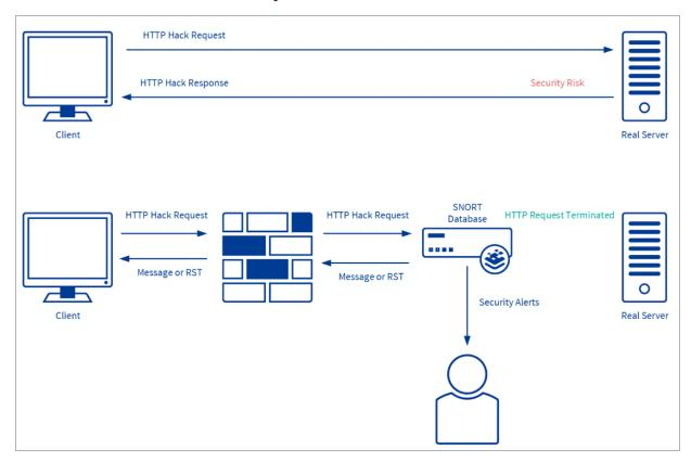
The LoadMaster is an established, hardened Internet appliance with HTTP intrusion prevention. In addition to Secure Socket Layer (SSL), Denial of Service support offered by the LoadMaster, the Intrusion Prevention System (IPS) service will provide in-line protection of Real Server(s) by providing real-time mitigation of attacks and isolation of Real Server(s). Intrusion prevention is based on the industry-standard SNORT database and provides real-time intrusion alerting.
