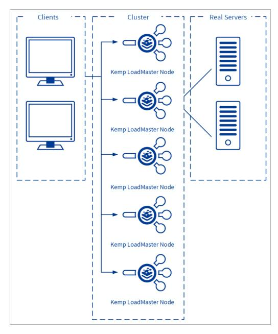
With LoadMaster clustering, the load-balancing capability can be extended as needed by adding additional LoadMasters for the same Virtual Service. Traffic which is intended for a failed node is either passed on to an existing node or load-balanced across the remaining nodes.
