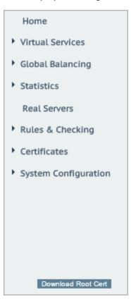
In order to eliminate this warning, the LoadMaster certificate can be installed by clicking the **Download Root Cert** button in the main menu on the **Home** page, when you first access the WUI in a browser.
