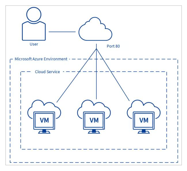
Any workload being published consists of an availability set, which represents a single VM or multiple VMs. When a VM is created, if an availability set exists, you have an option to connect the VM to an existing availability set. As more VMs are connected to an existing VM (and thus to an existing availability set), the built-in Microsoft Azure load balancer distributes connections when creating a load-balanced endpoint.
