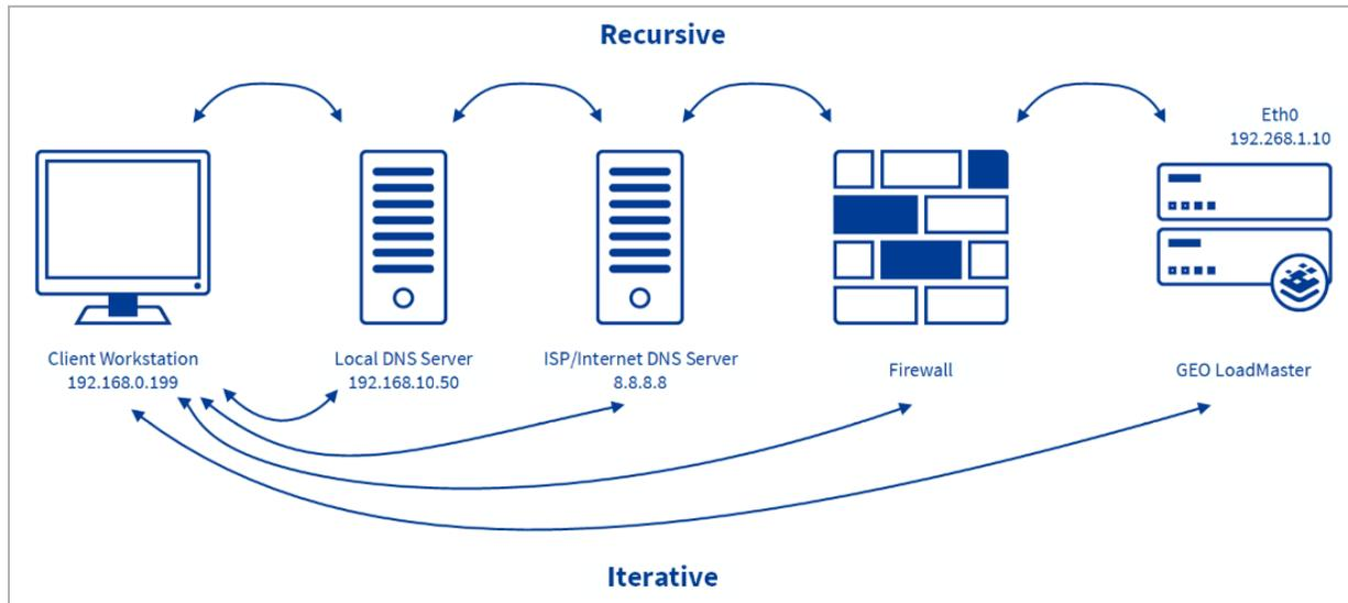
The above diagram illustrates the difference between recursive and iterative DNS.
