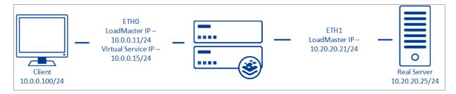
When **Subnet Originating Requests** is enabled, the Real Server sees traffic originating from 10.20.20.21 (LoadMaster eth1 address) and responds correctly in most scenarios.
