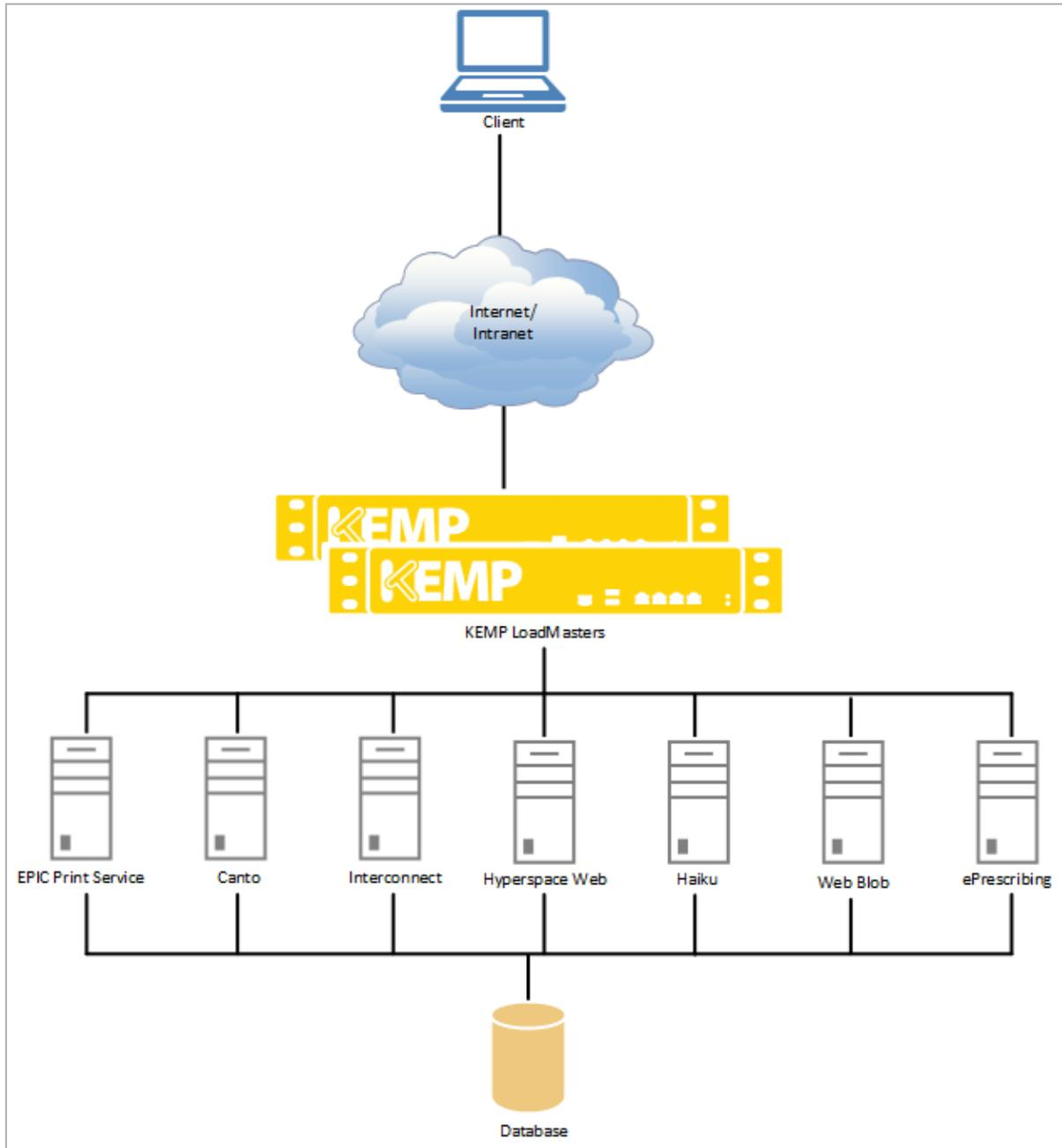
The above network architecture diagram depicts how the LoadMaster connects to the different backend components in Epic Systems.
