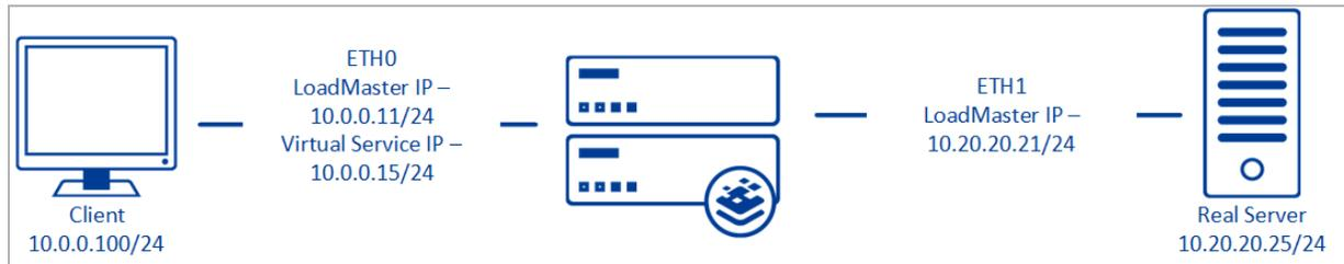
When **Subnet Originating Requests** is enabled, the Real Server sees traffic originating from 10.20.20.21 (LoadMaster eth1 address) and responds correctly in most scenarios.
