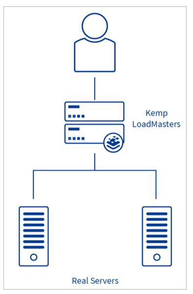
The LoadMaster offers advanced Layer 4 and Layer 7 server load balancing, SSL Acceleration, and a multitude of other advanced Application Delivery and Optimization (ADC) features. The Kemp
