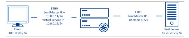
When **Subnet Originating Requests** is enabled, the Real Server sees traffic originating from 10.20.20.21 (LoadMaster eth1 address) and responds correctly in most scenarios.
