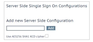
In the Server Side Single Sign On Configurations section of the Manage SSO screen, there is a check box called Use AES256 SHA1 KCD cipher. When this check box is selected, the AES256 SHA1 KCD cipher is used (by default the RC4 cipher is used).
