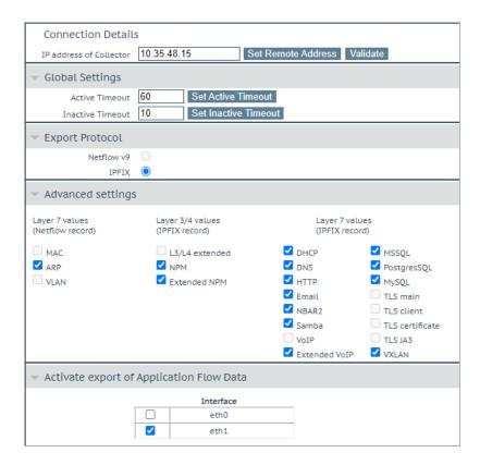
After you successfully install network telemetry on the LoadMaster, you should see a number of fields to configure on the **Network Telemetry** screen. Details on each of these options are below:
