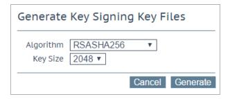
On the generate screen, select the cryptographic Algorithm and Key Size.
