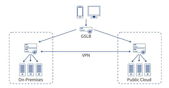
Figure 1- LoadMaster Hybrid Topology
