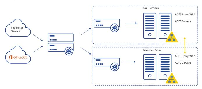
Kemp LoadMaster<sup>™</sup> delivers both the server and site resilience required to ensure that users have uninterrupted access to federated services in the event of an outage. The failover and recovery is totally automatic and transparent to the user community and requires no intervention from IT administration.
