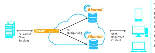
In the Akamai network infrastructure content services users contact the Akamai Edge Server which will either serve up cached content or place a call into the appropriate origin server. In the case where the Edge Server calls the origin server for content, there are two functions that the Edge performs that can complicate the operation of Load Balancers front-ending the infrastructure resulting in connection issues due to failed session persistence.
